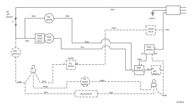
HARVEST-1 CYCLE (Hold Switch In Normal Position)
